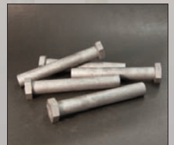
media blasted and descaled
