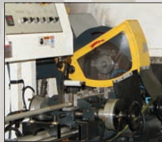
Bars are cut to length on our fully-automated bar saw.
