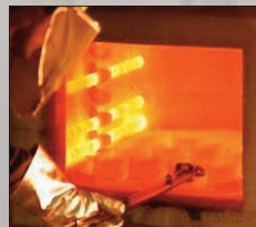
Headed blanks are heat-treated,
